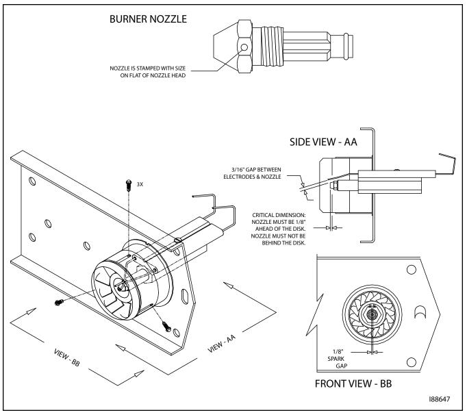
Figure 3H - Burner Nozzle and Electrode Specifications
