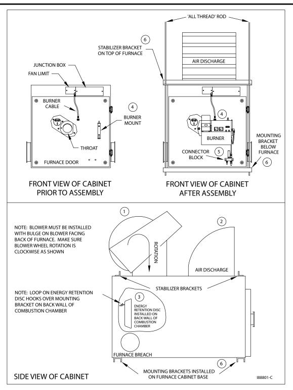
Figure 3A - Overview of Furnace Assembly
