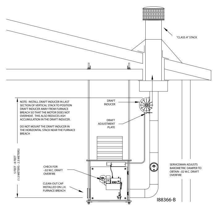
Figure 4R - Installation of the Draft Inducer
