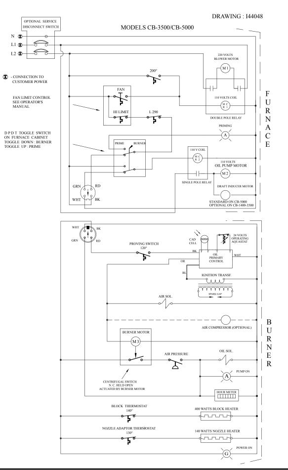
Figure B3 - Ladder Schematic for Models CB-3500/CB-5000 (220/240 Volts / 60 Hz)
