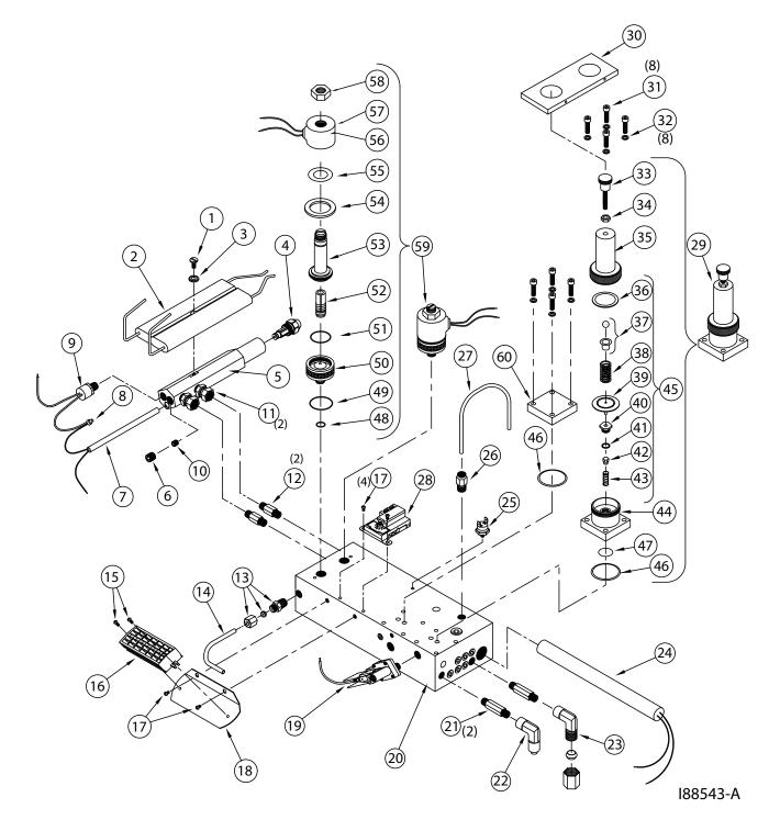
Figure A3 - Preheater Block Assembly Component Detail
