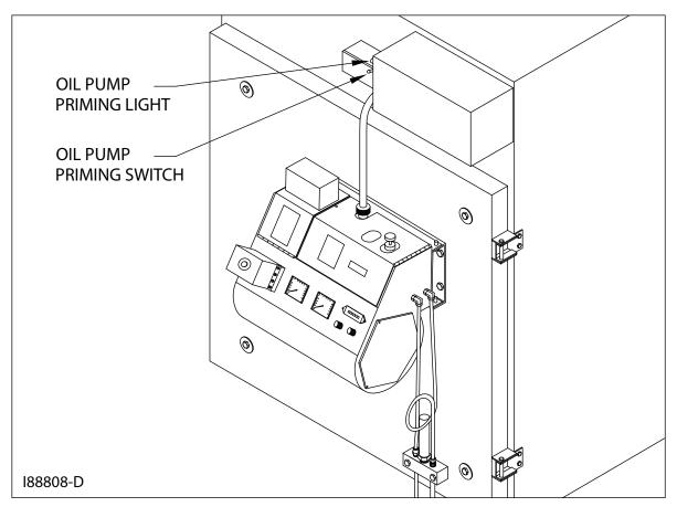
Figure 5B - Locating the Pump Priming Switch
