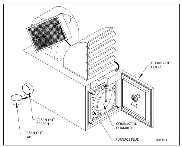
Figure 9E - Accessing the Combustion Chamber for Cleaning
