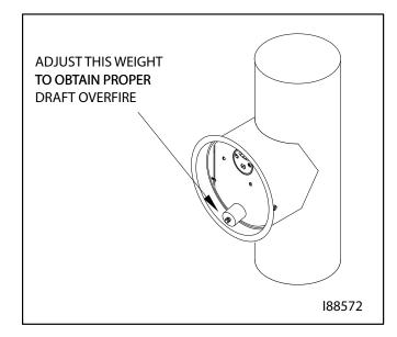
Figure 8B - Adjustment of Barometric Damper
