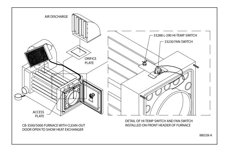
Figure 7B - Locating the F-180 Fan Switch amd the L-290 Hi-Temp Limit Switch
