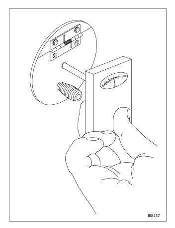
Figure 8A - Checking for Proper Draft Overfire
