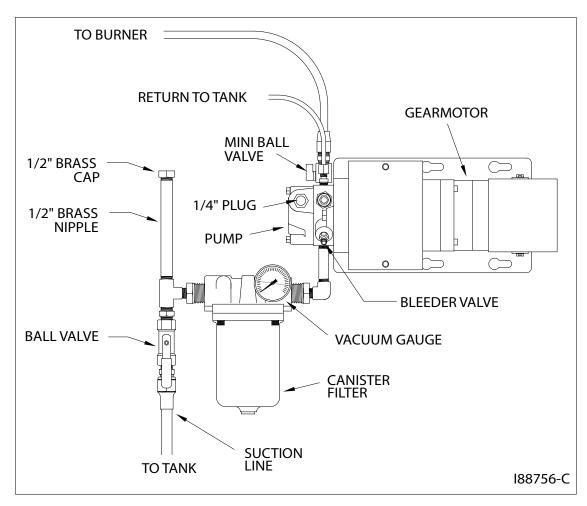
**Figure 5A - Priming the Metering Pump**
