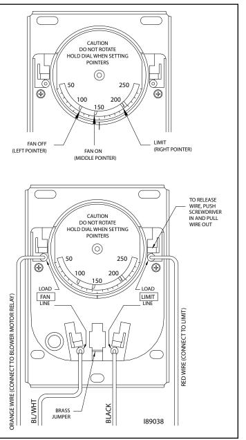
Figure 7C - Fan Limit Control Components
