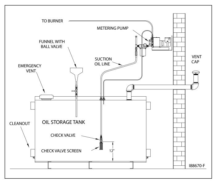
Figure 9D - Check Valve Detail
