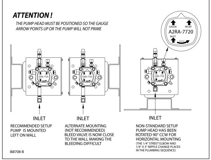
Figure 4I - Proper Positioning of Metering Pump Head
