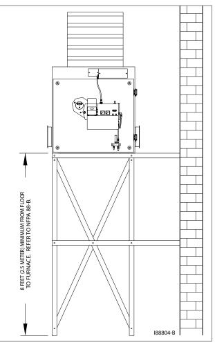
Figure 4D - Furnace Installed on Raised Platform
