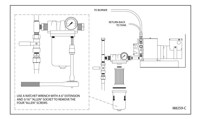
Figure 9B - Canister Filter Component Detail
