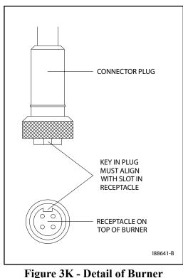
Figure 3K - Detail of Burne Electric Receptacle
