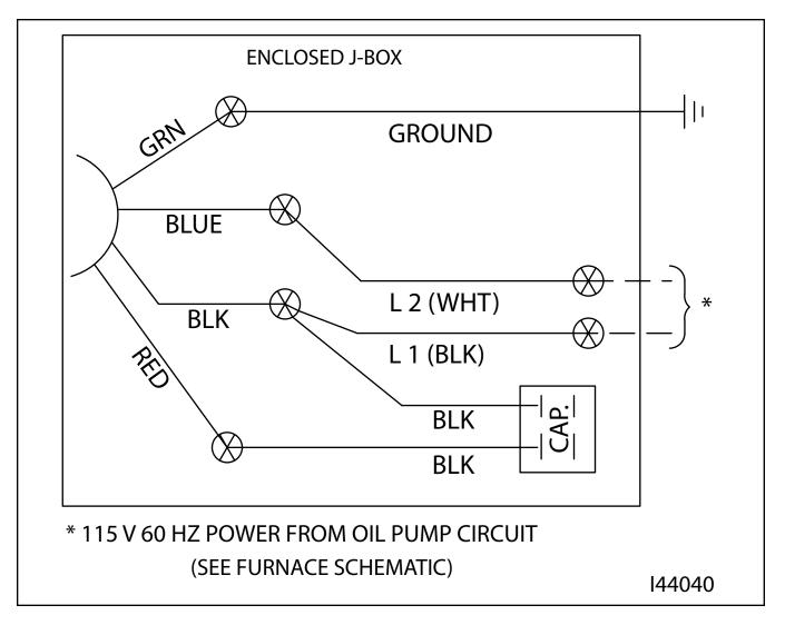
**Figure B4 - Metering Pump Wiring Schematic**
