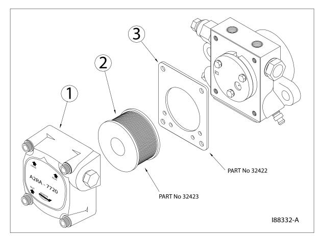
Figure 9C - Servicing the Metering Pump
