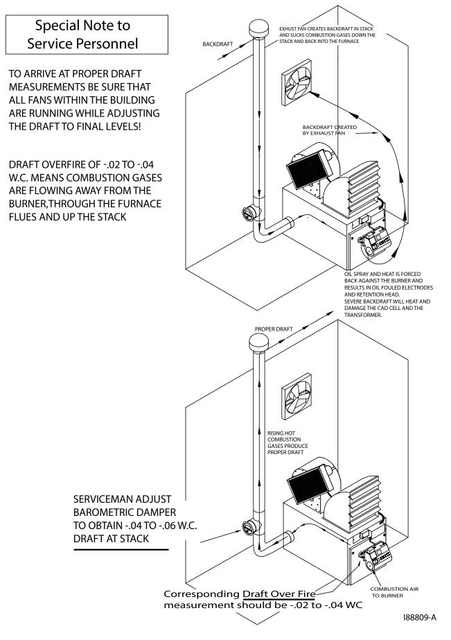
Figure 8C - Proper Draft vs. Backdraft
