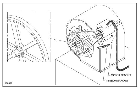
Figure 3E - Blower Assembly Installed on Furnace Cabinet
