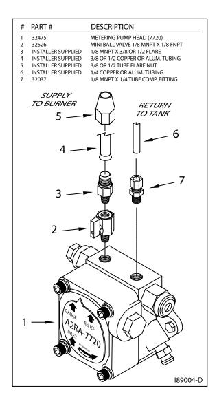
Figure 4K - Pressure Relief Oil Line Back to the Tank
