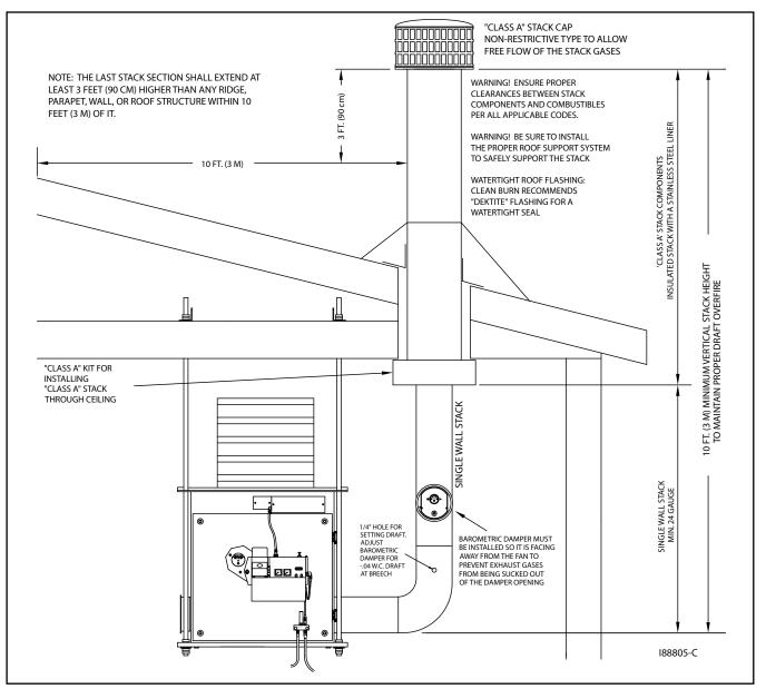
Figure 4C - Ceiling Mounting Installation Overview
