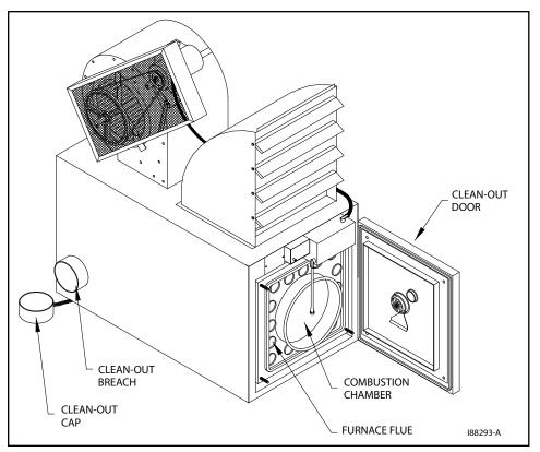
**Figure 2A - Accessing the Combustion Chamber**
