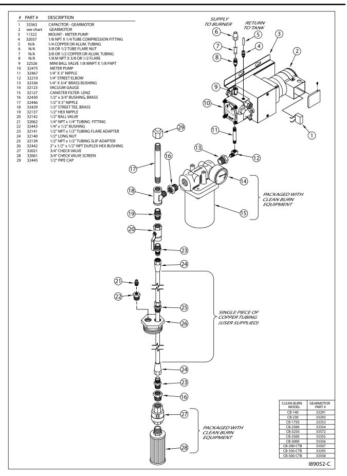
Figure 4H - Metering Pump Component Detail
